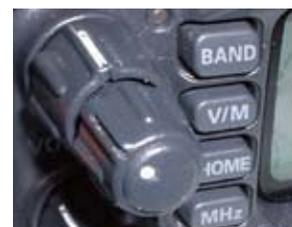
*Concentric controls on a Yaesu FT-7100m highlighted with Liquid Paper.*
