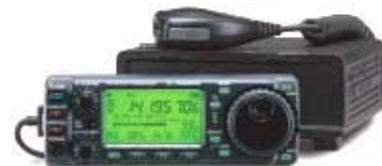
*The Icom IC-706 MkII is a small mobile radio covering 1.8 MHz to 440 MHz. Settings are changed through one of the five separate menus.*
