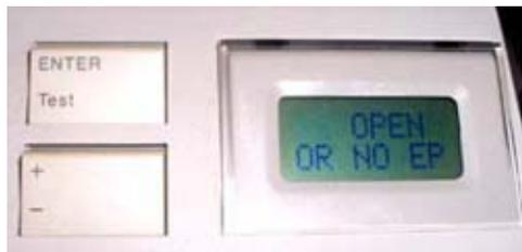
*Error message on the LaserJet IIP's control panel.*
