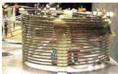
*Melted acrylic ribs from too much RF current.*
