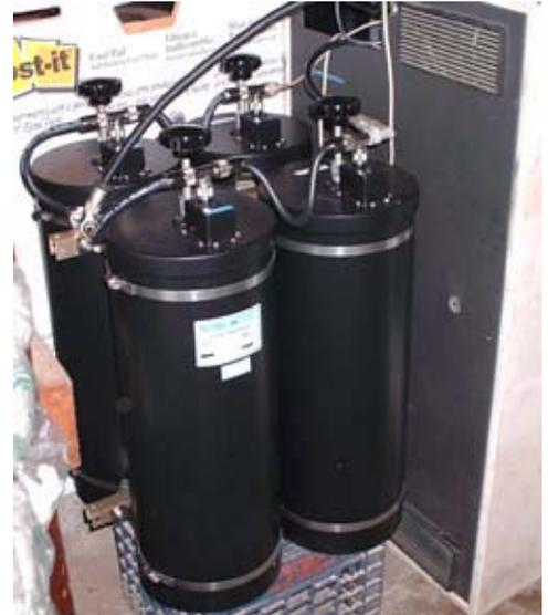
*Here's the brand new Decibel Products four cavity duplexer, alongside the Motorola Micor 2 meter repeater. Both are now under test in Bob, N2CBH's garage.*
