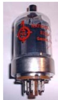
*The 6146B tube was often used in the final output stage of vintage HF transceivers.*
