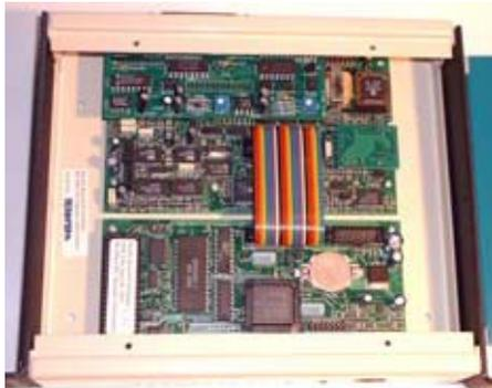
*View inside the new controller for the 2 meter repeater*
