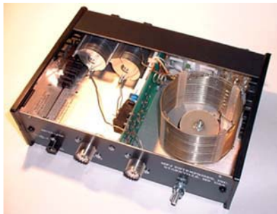
Antenna tuner containing reactive elements — variable capacitors and tapped inductors.
