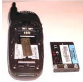
*Tiny 3.6V lithium-ion battery from a Motorola cell phone.*
