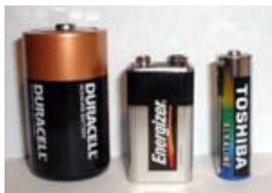
Three different sizes of alkaline battery — D, 9V and AA.
