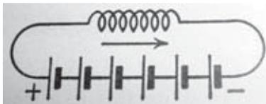
Six cells connected in series to form a battery.
