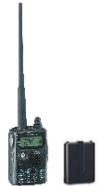
*Kenwood TH-F6A tri-band HT with 7.4 volt 1550mAh lithium-ion battery.*
