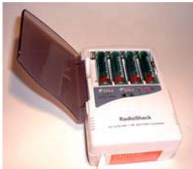
*Radio Shack 1-hour battery charger for nickel-cadmium and nickel-metal hydride cells.*
