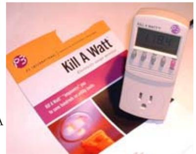
you can monitor the line voltage, the current drawn by the appliance, the power consumption in watts, the volt-amps (VA) draw, as well as the power-line frequency (Hz) and power factor. The line voltage and current are shown as true root-mean-square (RMS) values, rather than the calculated-from-mean figure of a typical inexpensive multimeter. There is also display of cumulative kilowatt-hours and elapsed time.
