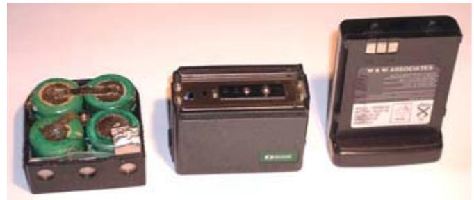
Three rechargeable nickel-cadmium batteries for different portable transceivers. The first battery case has been opened to show the individual cells.
