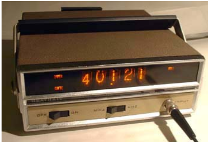
Here's the G3VNQ counter from the 1970s period, it's a Heathkit IB-1101 100 MHz digital frequency counter with five Nixie tube display, available from 1972 to 1975.
