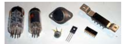
A mixture of vacuum tubes, transistors and chips (integrated circuits) from the '70s.
