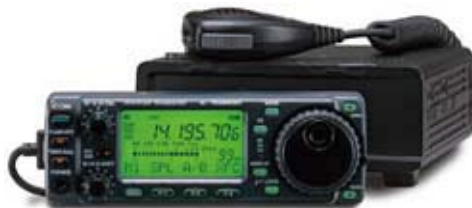
Icom's latest IC-706 Mk IIG transceiver includes 6 meters in its 1.8-450 MHz coverage.
