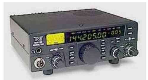
Ten-Tec model 526 "6N2" all-mode VHF transceiver, as used by N2CBH, covers six meters and two meters.
