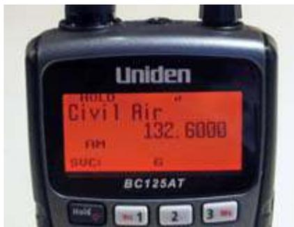
Successful reception of air-to-ground transmission on 132.600 MHz.
