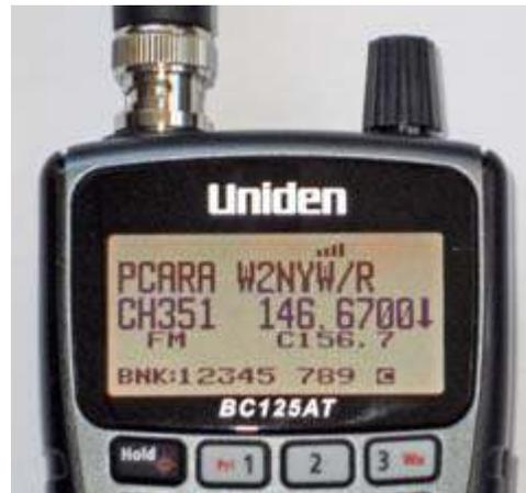
*Dot matrix display of the BC125AT shows signal strength, alpha tag, channel number, frequency, modulation mode, CTCSS (PL tone) and channel banks.*
