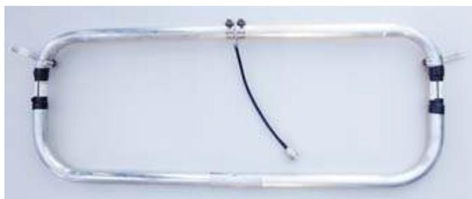
*Final form of Moxon Rectangle as built. The two hose clamps near the end-insulators are not structural, but add length to the driven element to lower SWR on the desired frequency.*
