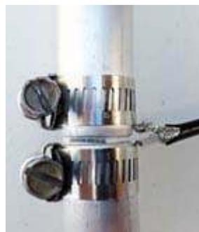
Driven element feed point showing the internal PVC pipe insulator and hose clamps holding the coaxial cable. [KD2ITZ pics.]
