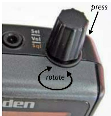
The BC125AT has a single rotary control which is used to **Select** a channel or menu item, **set the Volume** or **set the Squelch (Sql)**.
