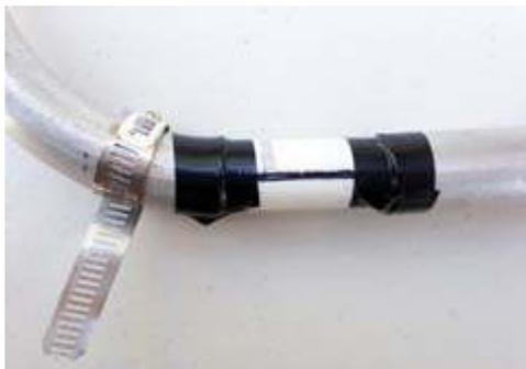
*PVC tubing end-insulator separates the driven element (left) from the reflector. Nearby hose clamp on the driven element was added to adjust resonance.*
