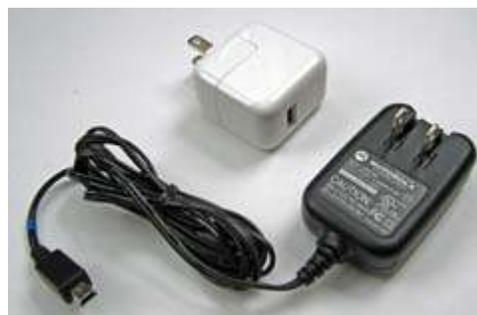
Apple iPod USB power adapter and Motorola phone charger with mini-B plug.
