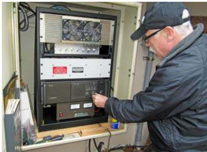
*Greg KB2CQE makes an adjustment to the Icom repeater's squelch control, completing November's improvements to the 449.925 MHz repeater.*
