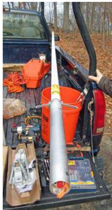
*Commander Technologies 1151-2N omnidirectional antenna is shown on the back of Bob's truck, after the radial kit was assembled.*
