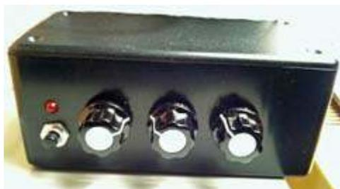
Rock-Mite QRP transceiver only has three knobs, one LED and a pushbutton.
