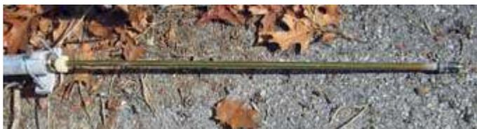
*The N-type coaxial connector with its attached radiating element had slid out of the base of the old Diamond X500 antenna.*
