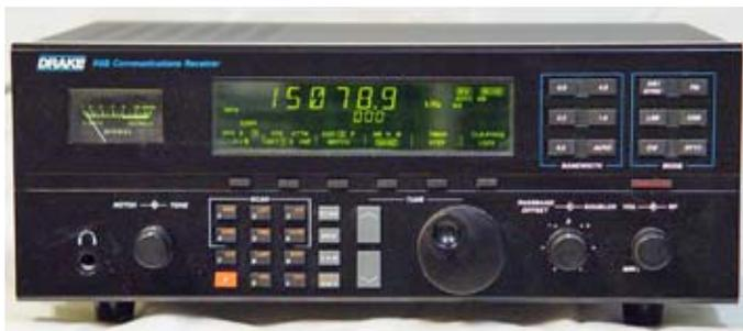
Drake R8B communications receiver covers 10 kHz to 30 MHz.
