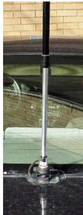
Close-up of Moonraker MD-7400 mobile antenna with the black plastic inductor tube raised to show the metallic mast that slides inside.
