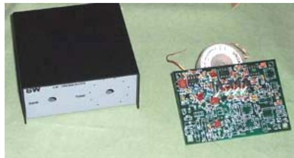
Small Wonder Labs SW+40 QRP transceiver kit, showing enclosure and circuit board.
