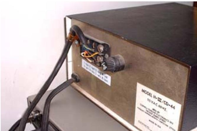
*Water must have run down the cable for the antenna rotator — seen here from behind.*
