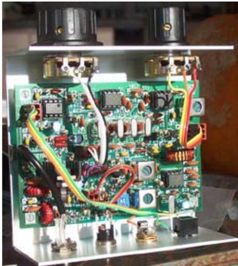
*View inside the SW+40, with the circuit board mounted in the enclosure.*
