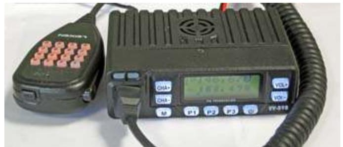
*Leixen VV-898 dual-band mobile transceiver only measures  $4\frac{3}{4}'' \times 1\frac{1}{2}'' \times 3\frac{3}{8}''$ .*
