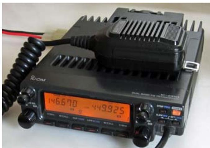
*Icom IC-2350H dual band transceiver.*
