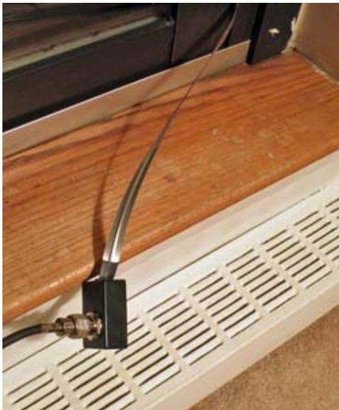
*Cable feed-through in use at W2CH.*
