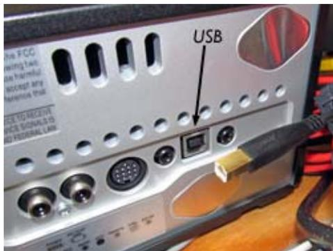
*USB type-B connector on rear of IC-7410 requires a USB A-B cable.*
