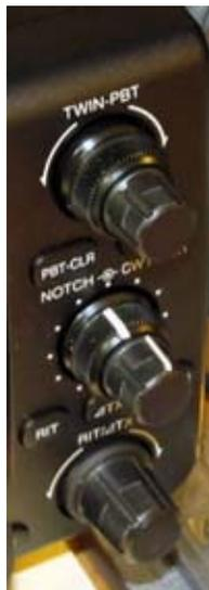
*Top to bottom — Twin pass band tuning control; Notch filter and CW pitch control; RIT and ΔTX incremental tuning control.*
