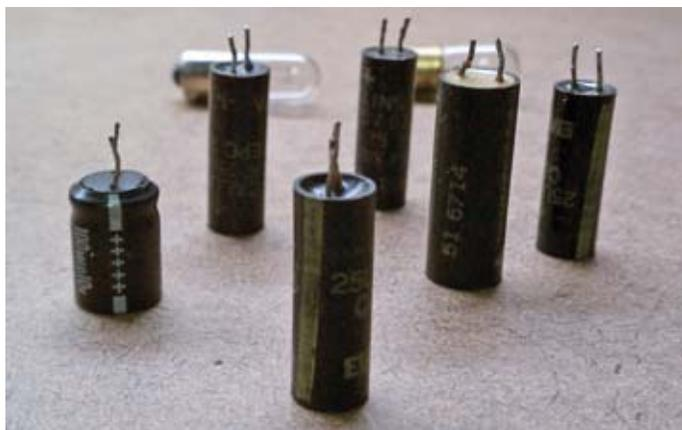
*Faulty capacitors removed from the receiver by Bob. In the background are some faulty bulbs.*
