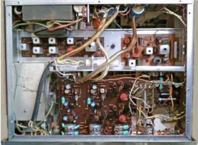
Receiver with the cover off, upper left is the IF and discriminator, upper right is the stereo decoder board, below is the audio board.
