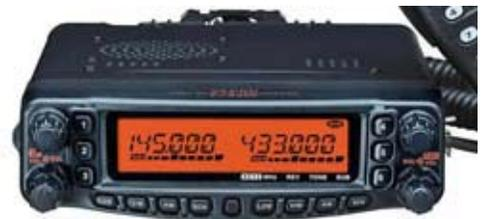
Yaesu FT-8800 dual band mobile transceiver.
