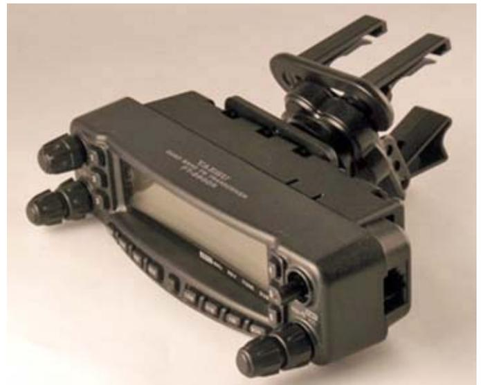
Remote head and bracket attached to a Lido LM-100 Vent Mount.
