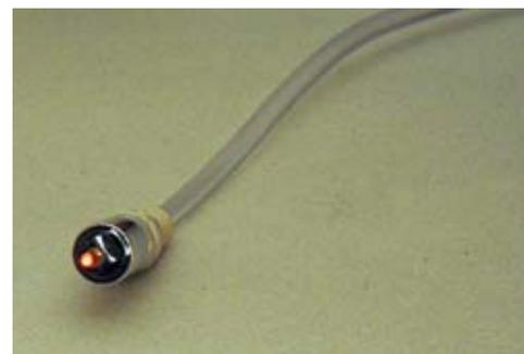
Clear TOSLINK plastic optical fiber cable for digital audio applications.
