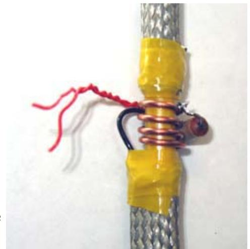
Matching coil at base of antenna. Coax inner conductor (black) is connected 3¼ turns up the coil — through a series capacitor for dual-band use. Twisted red insulated wire is the “gimmick” capacitor.
