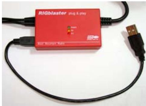
“RIGblaster plug & play” is a sound-card interface with USB connector for power and transceiver control.
