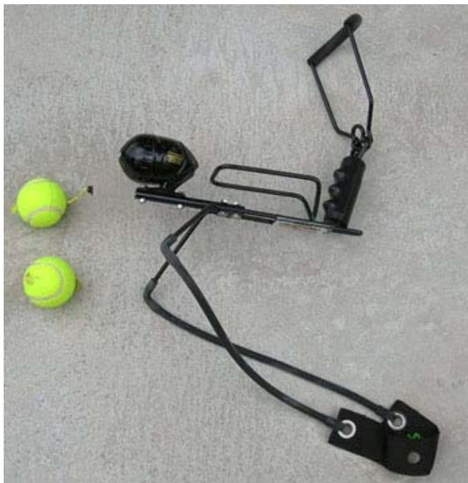
RadioWavz’ “Hyper Hanger” includes a Shakespeare Durango fishing reel, nylon line, Hyperdog sling and weighted tennis balls. [Picture by W2CH]
