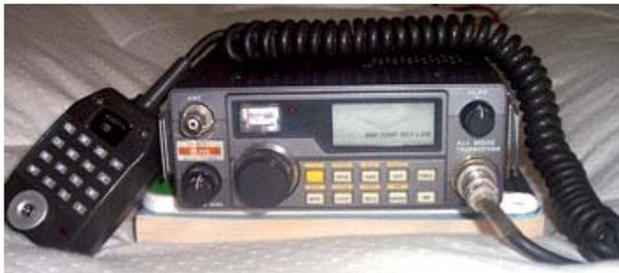
*Yaesu FT690R MkII transceiver for 6 meters covers 50-54 MHz with FM/SSB/CW modes at 2.5W output.*
