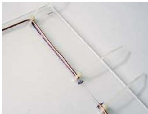
Detail of the 146 MHz Moxon built on a sheet of acrylic plastic, showing how the Moxgen and AC6LA calculators shown previously. My intention was to use nylon ties to hold the antenna wires in place, so I drilled pairs of holes (7/64") at the ends and at the corners of the wires. I used a small reel of 12 AWG copper/aluminum wire from A.C. Moore which was easy to bend and cut, folding the three lengths into shape then mounting them onto the acrylic sheet with nylon cable ties.
