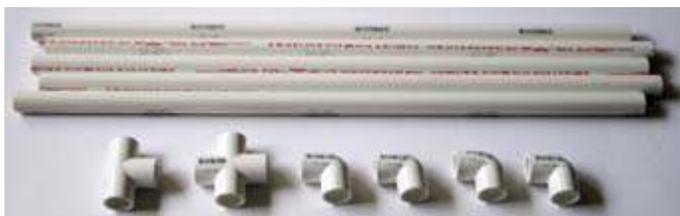
Raw materials for a Moxon — five lengths of 1/2 in. x 2 ft. PVC Sch. 40 Pipe, one tee, one cross and four 90° elbows.
