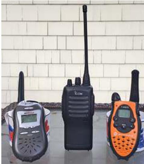
An FRS radio from Cobra (left) and an FRS/GMRS set by Motorola (right) alongside an Icom IC-F21GM (center). The IC-F21GM was considered the legacy standard GMRS/FRS handheld after its introduction in 2001.
