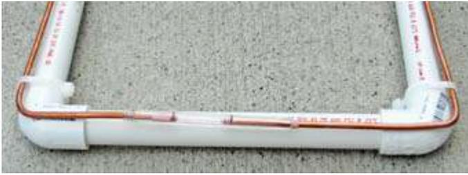
Close-up of 6 AWG copper wire fastened to PVC pipe with nylon ties. Element ends are inserted into a clear plastic ball-point barrel to maintain separation distance and alignment.
