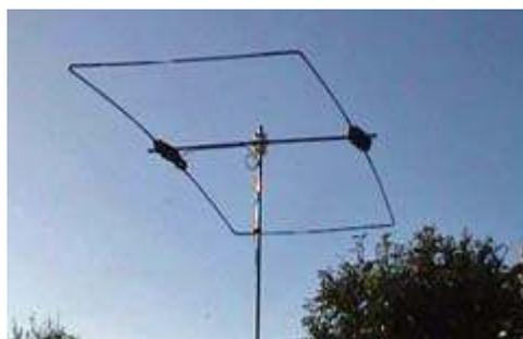
10 meter Moxon antenna built from 1/2" and 3/8" aluminum tubing by Mark, MOMRR. [Pic: Moxon Antenna Project.]
