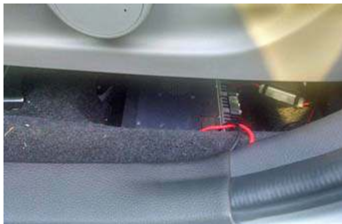
Yaesu transceiver is mounted under the driver's seat, with power and antenna cables routed underneath the plastic molding. [Pic - N2CBH]
