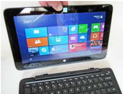
HP Pavilion x2 convertible notebook displaying the Windows 8 Start Screen. It can operate as a laptop with keyboard and touch-pad attached or as a touch-screen tablet when detached.
