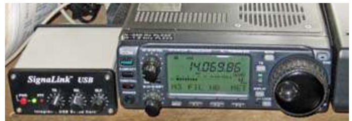
Signalink USB Sound Card adapter for digital modes connected to the Icom IC-706 MkII G transceiver .
