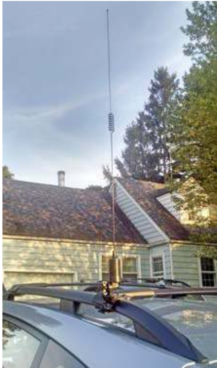
Larsen dual-band antenna on Diamond NMO mount, attached to Forester's luggage rack. [Pic - N2CBH]
