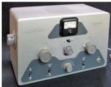
Heathkit DX-20 transmitter covered 80-10 meters, CW only.
