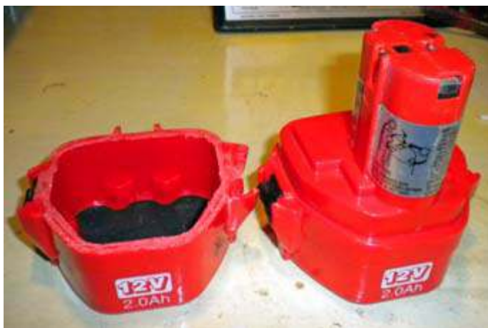
12 volt battery pack for Makita drill has been cut open and the NiCd cells removed (left). An unopened battery pack is shown on the right. [Pics - N2CKD]
