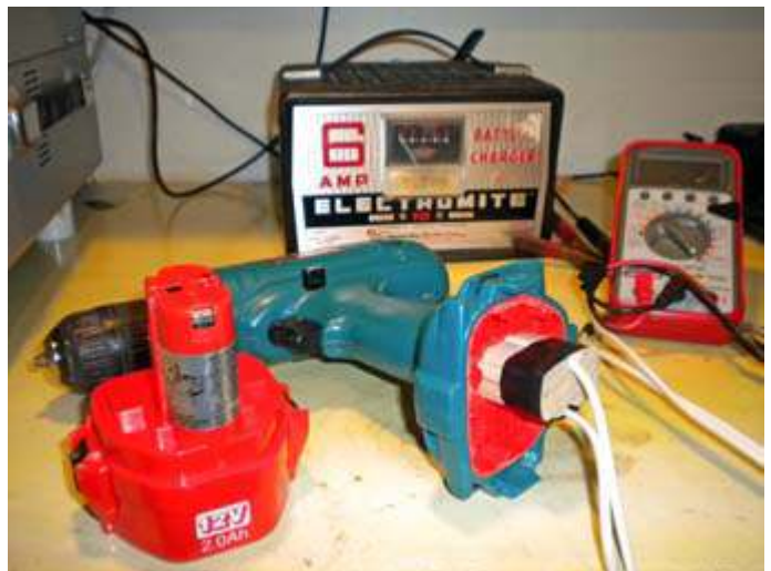
The modified battery pack was tested in the drill, using a 12 volt battery charger as power source. Lovji monitored current draw on the amps range of a VOM multimeter.
