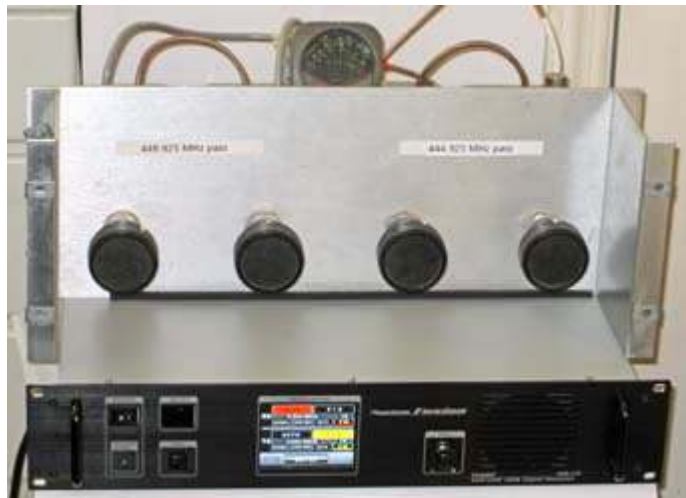
PCARA's DR-1X Fusion repeater operating in the test location, with antennas fed through the Motorola cavities.
