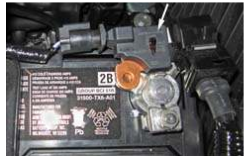
Bosch electronic load detector ( ELD ) attached to the negative terminal of a recent Honda vehicle's battery.
