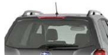
Subaru AM/FM 'duck' antenna located at the back of the roof.
