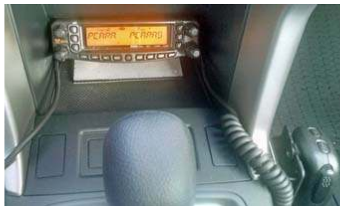
Close-up of the FT-8800R remote head, mounting bracket and microphone, fixed to the Subaru Forester's center console with Scotch Extreme fasteners. [Pic by N2CBH]
