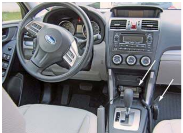
Bob mounted the FT-8800 remote head and microphone (arrowed) in the lower half of the Subaru center console.
