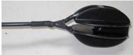
*Commercial antenna with PVC-insulated wire threaded through an egg insulator. Insulation has been removed from the wire so the end could be wrapped around exposed conductor and soldered. The soldered joint is covered with heat-shrink tubing for added strength and corrosion protection.*
