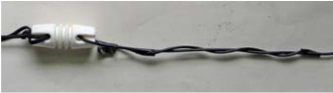
Wire antenna with excess wire threaded through the end insulator, folded back then twisted round itself.
