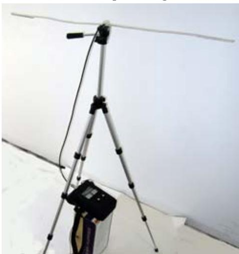
*Experimental set-up for measuring the resonant frequency of insulated wire antennas. The horizontal dipole is supported on a camera tripod and connected by coaxial cable to an MFJ-259 Antenna Analyzer.*
