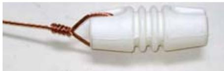
Antenna with bare copper wire threaded through the end insulator then twisted back on itself.
