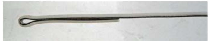
*Oversized dipole antenna made from PVC-insulated wire had its ends folded back for an overall length of 35¼".*
