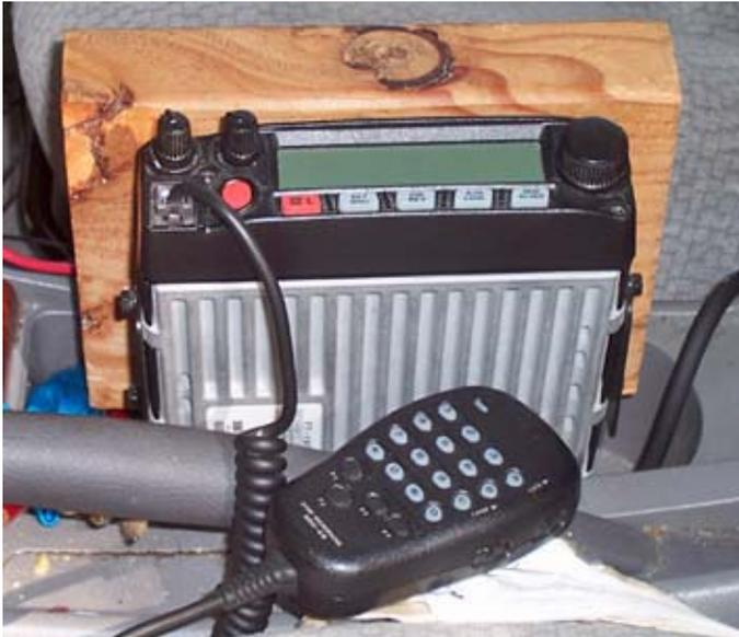
*Karl mounted his Yaesu FT-1900R transceiver on a wooden base, standing up in the Toyota's cup holders.*
