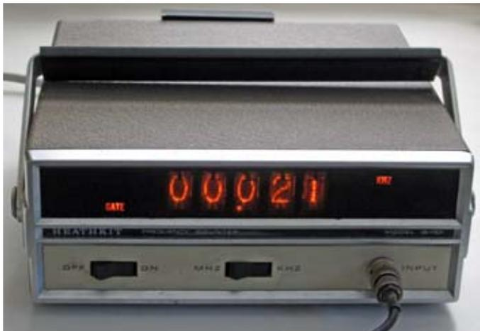
*My Heathkit IB-1101 frequency counter from 1973 has neon-based Nixie tubes in the display.*
