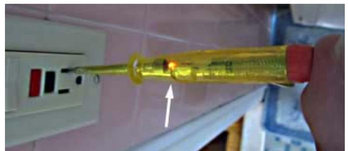
*Neon screwdriver glows dimly on 120 volts AC.*
