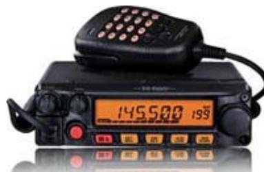
*Yaesu FT-1900R transceiver is a rugged, single band, 55 watt transceiver for 2 meters.*
