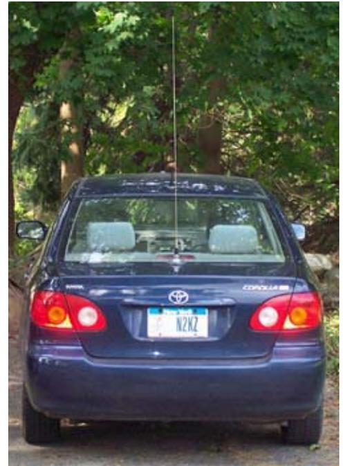
*Rear view of Karl's vehicle with newly-installed Diamond M285 monoband antenna for 2 meters.*
