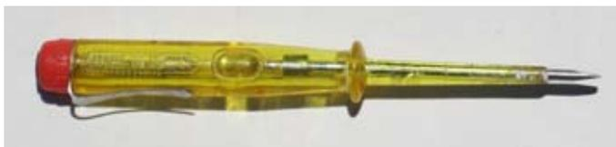
*Neon screwdriver combines a detector for high voltages with a traditional slotted screwdriver.*
