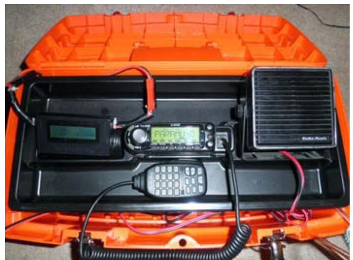
Top view of Ray's "radio in a box". Left to right are the Astro Flight Whattmeter 101, Icom ID-880H control head and Radio Shack external speaker. [Pic by W2CH]
