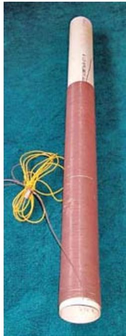
*Loading coil for MF wound on PVC pipe.*
