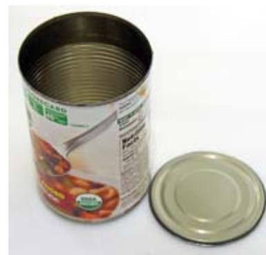
*Internal surface of a tin can is protected by an epoxy resin coat manufactured from Bisphenol A.*
