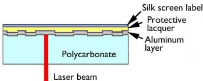
*The layers of an audio CD. Molten polycarbonate flows into the mould, forming pits and lands on the polymer’s top surface. This surface is coated with aluminum to reflect the laser beam shining from below. A protective lacquer layer is added to prevent scratches and corrosion. The label is then screen-printed in one or more colors.*
