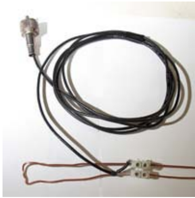
Coaxial cable connected to matching section using barrier strip block. Slide to adjust.
