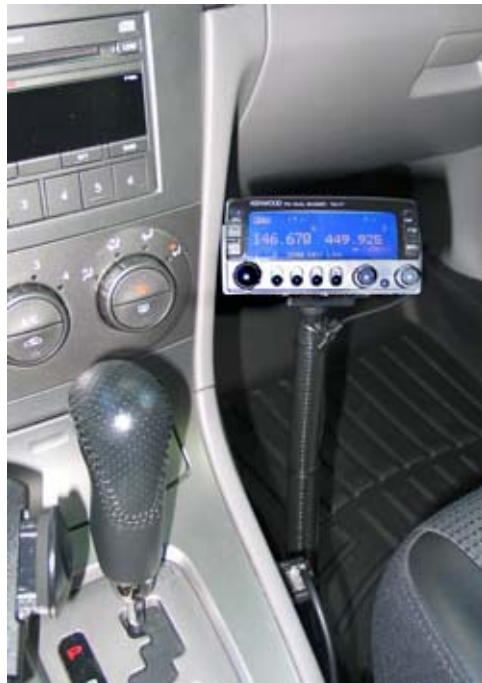
Kenwood TM-V7 control head, newly mounted in the KB2CQE vehicle.
