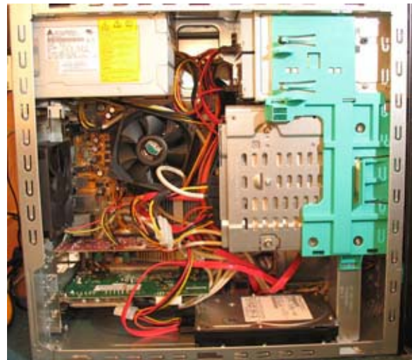
Inside the new PC. The thick red 'spaghetti' strands are SATA cables connecting the hard drives and DVD drives to the motherboard.
