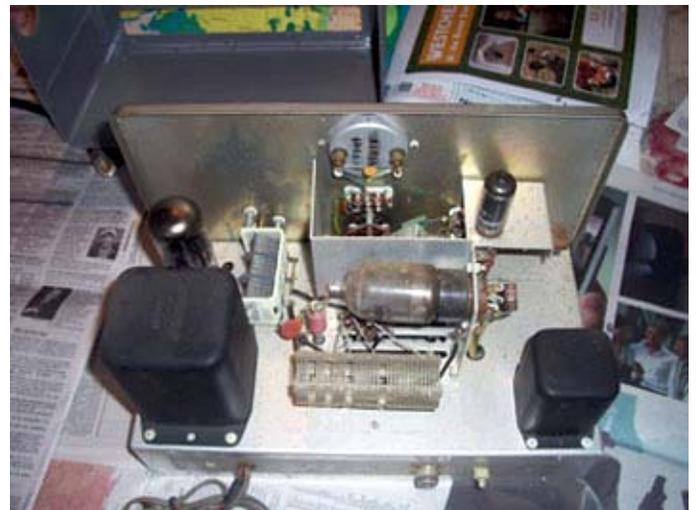
*Heathkit DX-20 has 5U4G double diode rectifier (left), 6CL6 VFO (right) and 6DQ6A PA (horizontal, center).*
