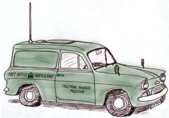
*Ford Thames van as driven by the U.K. Post Office Radio Service in the 1960s. The fiberglass whip antenna was connected to measuring equipment in the back of the vehicle.*
