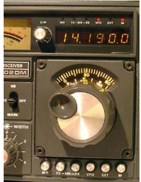
The FT-902DM frequency control drives a rotary tuning dial. The digital frequency display is above. To the left is the “Mark” switch for 100 kHz crystal calibration.
