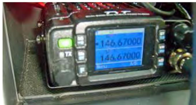
*TYT TH-8600 dual-band transceiver after completion of installation in Subaru Forester. [KD2EVI pic.]*
