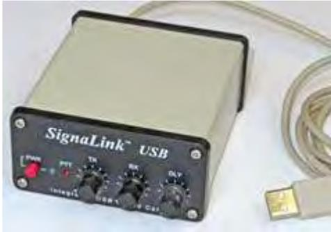
*Signalink™ USB interface connects transceiver audio to personal computer using its own built-in USB sound-card.*
