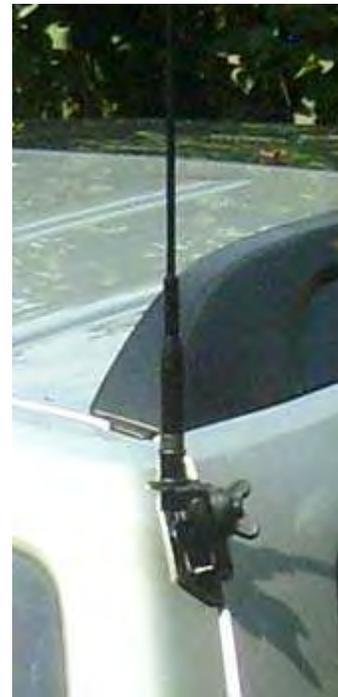
*Comet SBB-1 flexible, rubber-coated dual-band antenna with CP-5 lip mount, installed on Subaru tailgate.*
