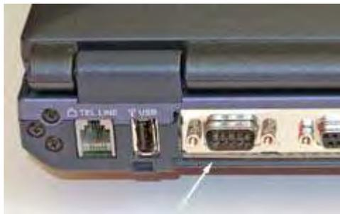
Old-style notebook has built-in serial port with DE-9 male connector (arrowed).
