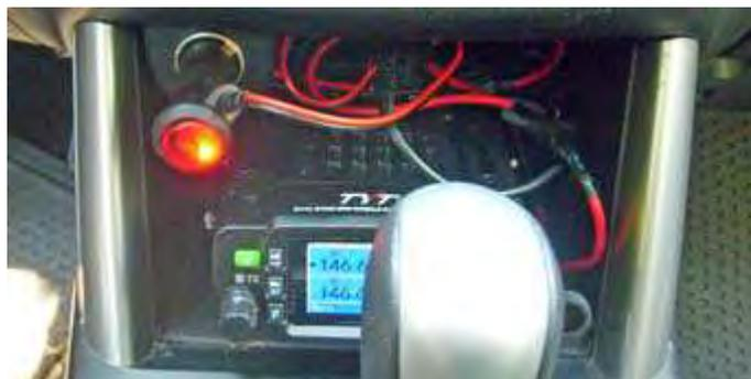
*TH-8600 power cord was soldered to an illuminated cigar lighter plug then connected to a nearby 12 volt outlet.*
