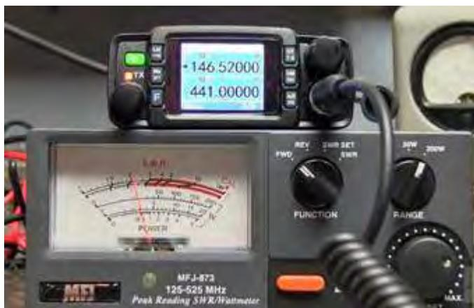
TYT TH-8600 power output was 21 watts on 146 MHz when measured by Jason, KC5HWB of 'Ham Radio 2.0'.
