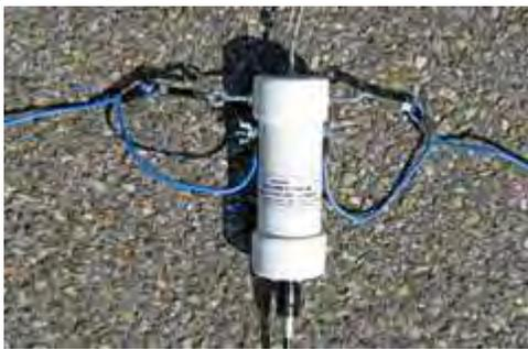
*Buxcomm OCFD Windom antenna with 4:1 balun at the off-center feed point.*
