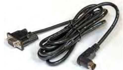
*Kenwood PG-5G PC programming cable connects 8-pin mini DIN socket on the back of a TM-V71A or TM-D710GA to 9-pin D-sub connector of an old-style PC’s serial port.*
