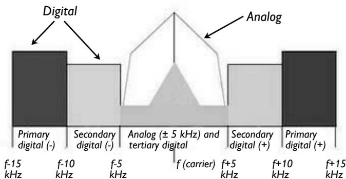
Diagram of IBOC HD Radio spectrum in hybrid AM mode. Analog sidebands are restricted to  $\pm 5$  kHz above and below the carrier frequency. Digital sidebands extend  $\pm 15$  kHz above and below the carrier.
