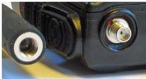
*Yaesu FT-70DR has a female SMA antenna connector at the top of the radio (right) and a male connector in the base of the stock YHA-72 antenna.*
