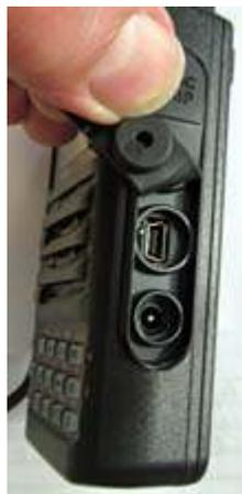
*Mini-USB connector and charging socket are on the radio’s right side.*
