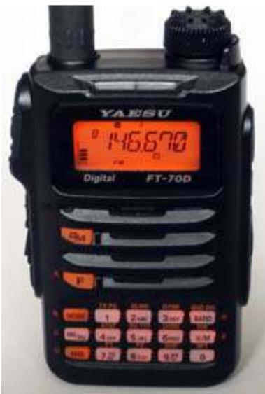
*Red backlight illuminates the liquid crystal display and all the front panel buttons.*
