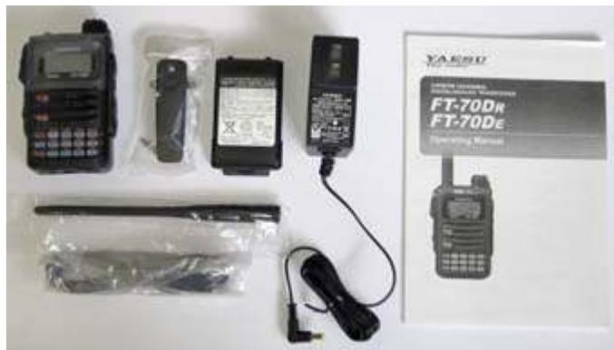
*Items included in the FT-70DR box, L to R: radio body, belt clip, lithium-ion battery, AC charger, Operating Manual. Below are the antenna and USB data cable.*
