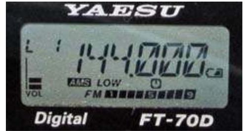
*Close-up of the liquid crystal display shows volume setting at left and nine bars of the S-meter below the frequency read-out. Symbol on right shows battery voltage OK.*
