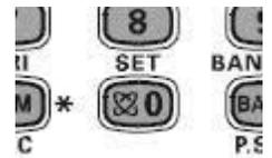
*‘WIRES’ key on the SET/0 button of the Yaesu FT-60R.*
