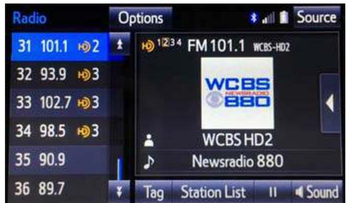
WCBS-FM on 101.1 MHz carries the audio of WCBS-AM (880 kHz) on its HD2 digital subchannel.
