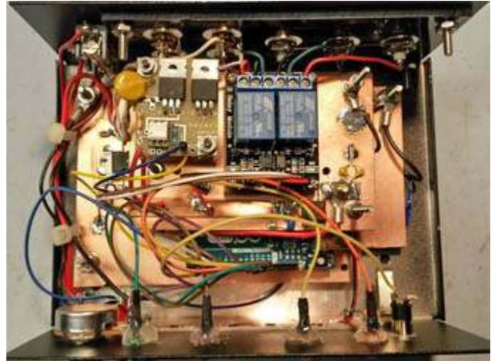
*Interior view of the T-R Time Machine. The Arduino microcontroller board sits below the Keyall HV board (top left) and the Arduino two-relay module (top right).*
