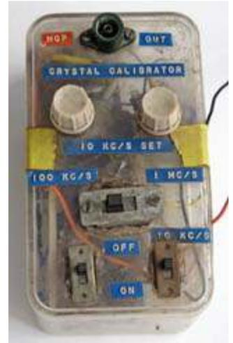
Crystal calibrator was not pretty but it did produce harmonics of 1 MHz and 100 kHz. Note ‘kc/s’ on the embossed Dymo labels.
