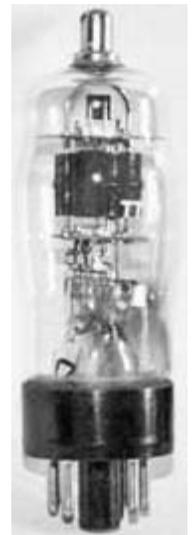
TT11 tube as used in power amplifier (PA).
