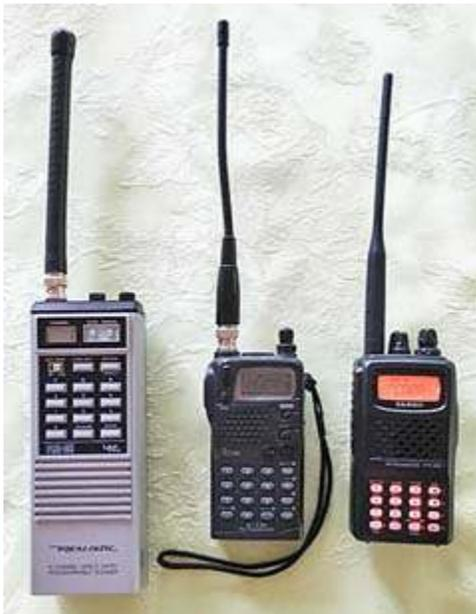
Three items from Karl's chronicle of hand-held amateur radio devices. On the left is a Realistic PRO-38 scanner which Karl first listened with. In the center is the Icom IC-T7H dual band handi-talkie which gave many years of service. On the right is the latest acquisition — a Yaesu FT-60 HT.
