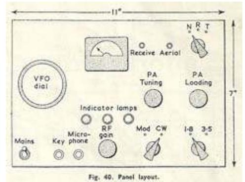
Fig. 40. Panel layout. Front panel layout for the low power 160 meter transmitter.
