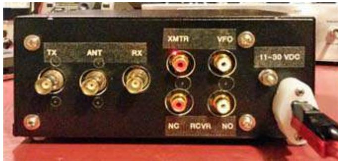
Back panel of the T-R Time Machine. Jacks are mounted on a plastic panel behind the aluminum enclosure from LMB Heeger, <http://lmbheeger.com/interlockingseries.aspx>.
