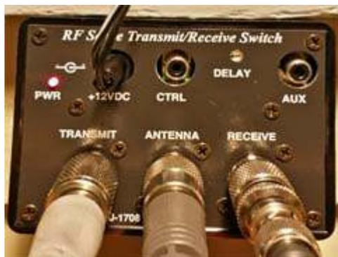
*MFJ-1708 RF-sensing Transmit/Receive Switch changes the antenna over from a separate receiver to the transmitter and handles 200 watts PEP.*
