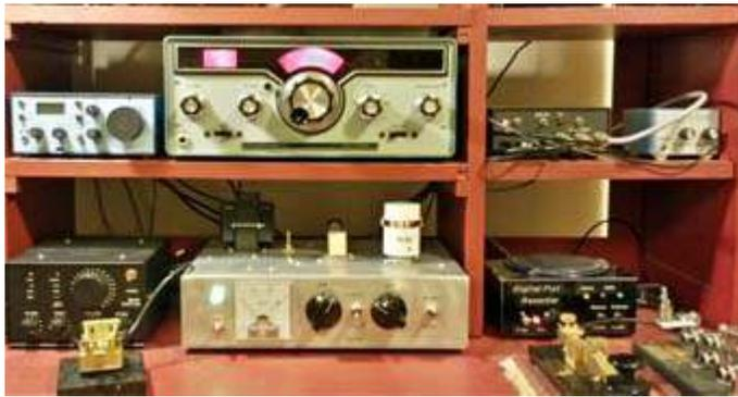
The Heathkit HR-1680 CW/SSB receiver (top center) for 80-10 meters fits nicely into the upper shelf of Mike's QRP equipment stack.
