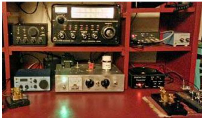
*The Drake 2B receiver (top center) was fitted into Mike's QRP stack by removing one of the shelves. The basic Drake 2B covers the 80, 40, 20, 15 and 10 meter amateur bands in 600 kHz segments.*
