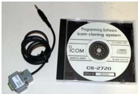
*Icom OPC-478 serial cable plus Icom's programming software on CD-ROM for the IC-2720 FM transceiver.*
