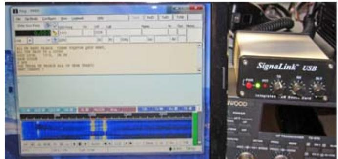
*Screen-shot of FLDIGI receiving RTTY alongside the Signalink USB radio interface.*
