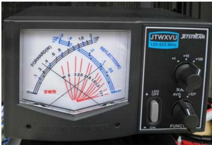
Jetstream JTWXVU VHF/UHF power and SWR meter
