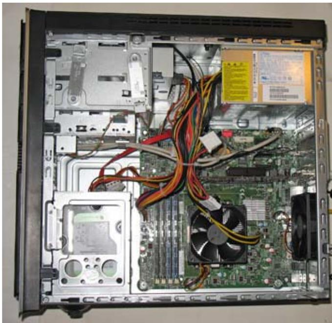
*Inside the new PC. The four-core AMD processor is underneath the fan.*
