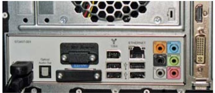
*Connections on the rear of the new PC. Round PS/2 connectors for keyboard and mouse have been replaced by two more USB ports (bottom left). VGA connector for the display has been replaced with HDMI ((High-Definition Multimedia Interface) or DVI (Digital Visual Interface) connectors (right).*
