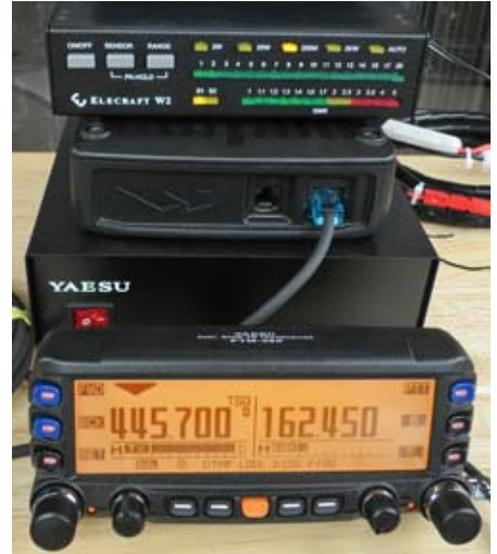
Ray's test setup for the VHF/UHF power meters, using a Yaesu FTM-350R mobile transceiver as the RF source.
