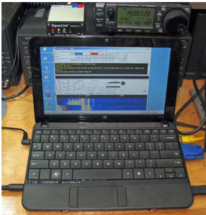
Netbook computer is shown receiving PSK-31 signals on 20 meters using Hamscope software. Sound card audio is connected through a SignalLink SL-1 radio interface to the Icom 706 MkIIg transceiver.
