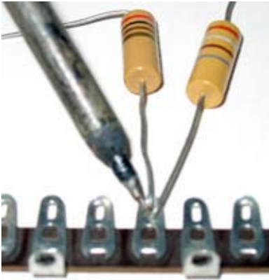
How to solder well — Step 1. first heat the component leads with the tip of the iron.
