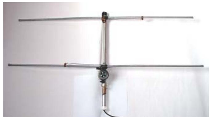
HB9CV antenna for 2 meters. The gamma match/phasing line is connected to the elements with copper clamps. A magnetic compass is attached to the boom for bearings.
