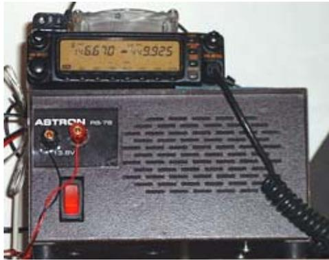
*PCARA IRLP node # 4214 now makes use of a Yaesu FT-8000 transceiver. The small 12 volt cooling fan on top is run from 9.4 volts for low noise.*
