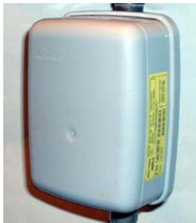
*Neptune R900 Meter Interface Unit transmits the meter reading to a passing vehicle using the 910-920 MHz frequency range. This is the wall-mount model.*
