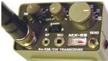
*Santec MX-6S 6 meter QRP transceiver was made by Mizuho and has 1 watt output on SSB or CW.*
