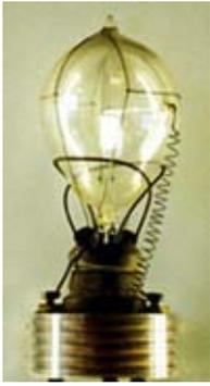
Fleming valve - the first electron tube.
