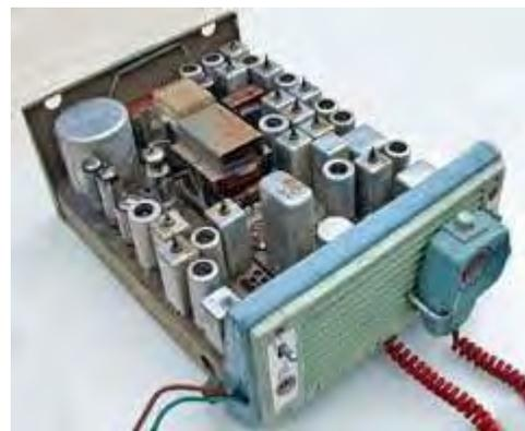
Pye Ranger mobile radiotelephone had vacuum tube transmitter and receiver.
