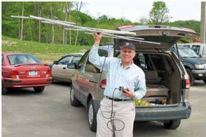
Karl demonstrates his 4-element Yagi antenna with PVC handle during the PCARA Foxhunt of May 2006.
