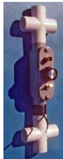
Active attenuator incorporated into boom of a tape-measure Yagi.
