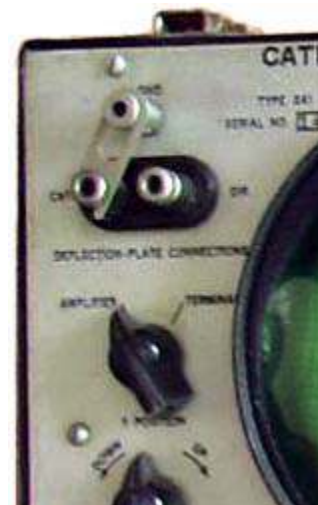
Dumont 241 vertical deflection plate terminals.
