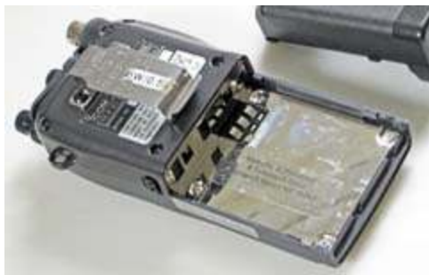
Find yourself a handi-talkie with a metal case — otherwise strong signals can leak into the case and you will need an offset attenuator.
