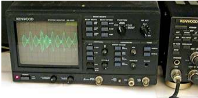
Kenwood SM-230 station monitor displays waveform of an outgoing 14 MHz SSB transmission from the adjacent Kenwood transceiver.
