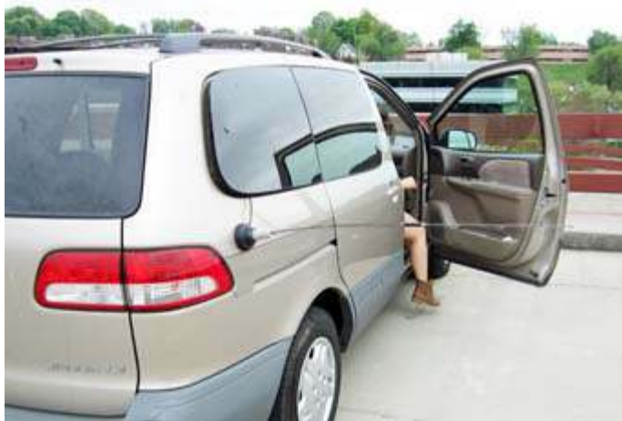
The fox could be using a horizontally polarized mag-mount antenna on the side of a vehicle. [May 2015.]
