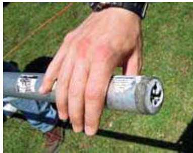
The threaded coupling which projected from the end of this aluminum tube had sheared off.
