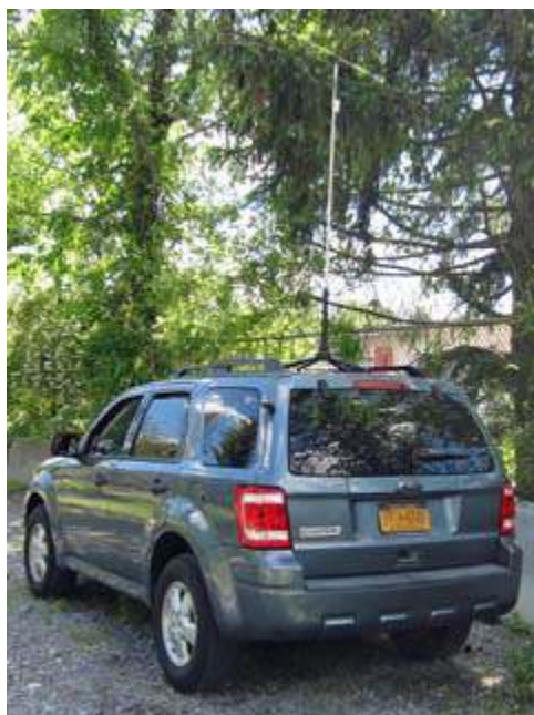
Close-up of the fox vehicle and antenna. Horizontal transmit dipole for 146 MHz is just visible on top of the fiberglass pole.
