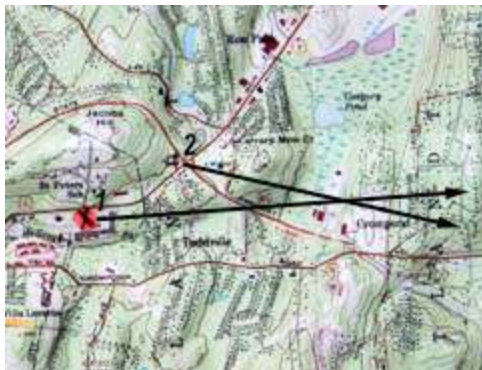
From position '2', make a new line on the map in the direction of maximum signal then head to where the two lines cross.
