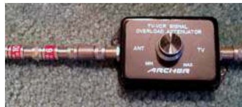
Karl's adjustable TV/VCR signal overload attenuator in series with 6dB and 10dB fixed attenuators.
