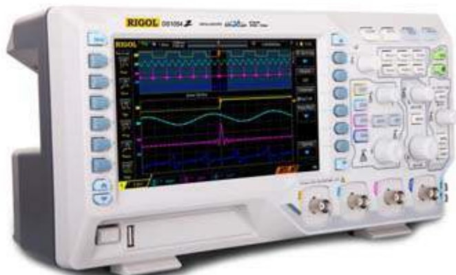
The Rigol DS1054Z is a popular digital oscilloscope from China with 50 MHz bandwidth and four input channels.
