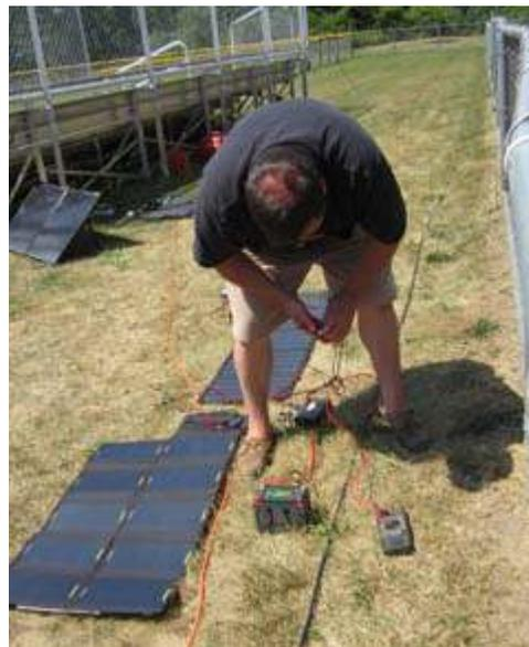
Mike W2IGG checks the state of a 12 volt lithium battery as it is being charged by nearby solar panels.
