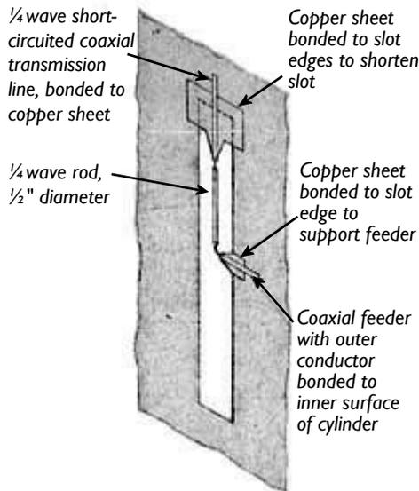
Coaxial feed arrangement for an individual slot of the Wrotham FM antenna system.
