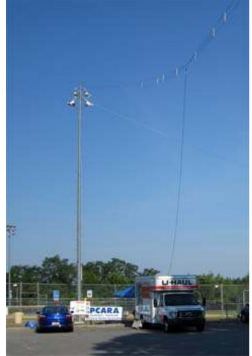
Multi-band dipole for 10, 15, 20 and 40 meters and part of the G5RV antenna are just visible, suspended from the top of the same light pole.
