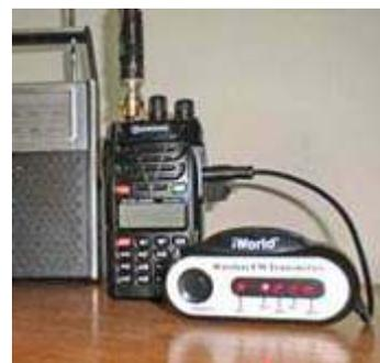
Personal FM transmitter sends audio from a 2 meter HT to the larger speakers of a nearby FM receiver. [N2CKD pic.]
