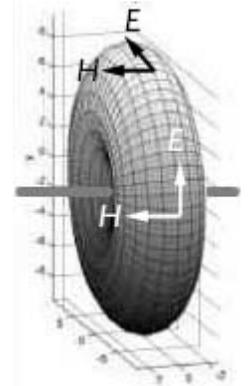
Electric (E) and magnetic (H) fields for a horizontal slot antenna cut into a vertical sheet.
