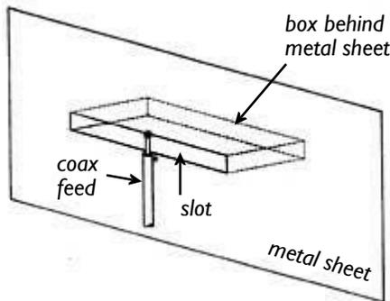
Boxed-in slot antenna radiates on one side of the sheet only.
