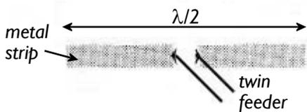
When the strip of metal removed from the slot antenna is fed in the middle, it produces the 'complementary antenna'.
