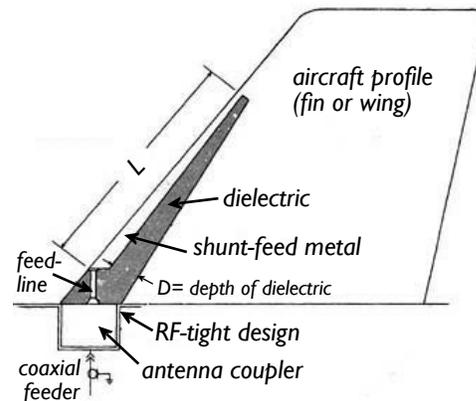
Collins notch antenna for HF use on aircraft is shunt-fed across the open end. Dielectric material can be fiberglass.
