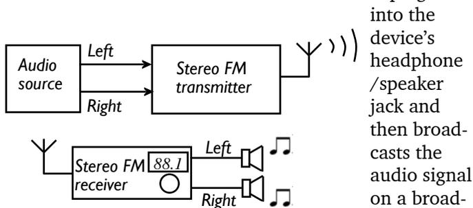
Diagram shows a low-power FM transmitter being used to couple the output from an audio device to a nearby stereo FM receiver.
