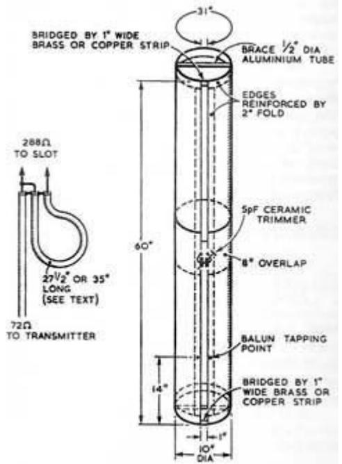
Cylindrical slot antenna for 2 meters with suitable balun (left) as described in RSGB publications.
