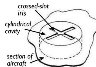
Boeing cavity-backed slot antenna for satellite work.
