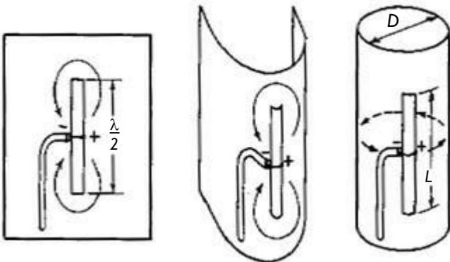
Transformation of a vertical sheet with a slot into a slotted cylinder (after Kraus - Antennas). Once the edges meet to form the cylinder, currents can circulate *behind* the slot.
