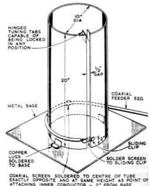
Abe Lincoln mobile antenna for 144 MHz is open at one end (notch antenna).
