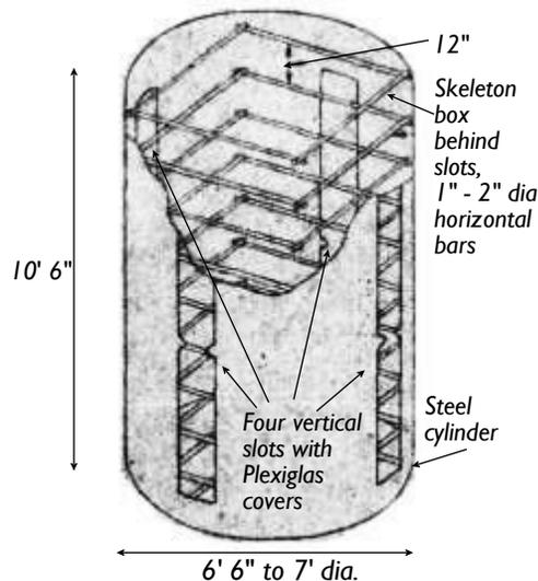
Structure of one tier of the eight-tier slot antenna employed by the BBC at Wrotham.
