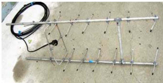
J-Beam 8-over-8 skeleton slot antenna for 430 MHz suffered several bent elements on its trip across the Atlantic.
