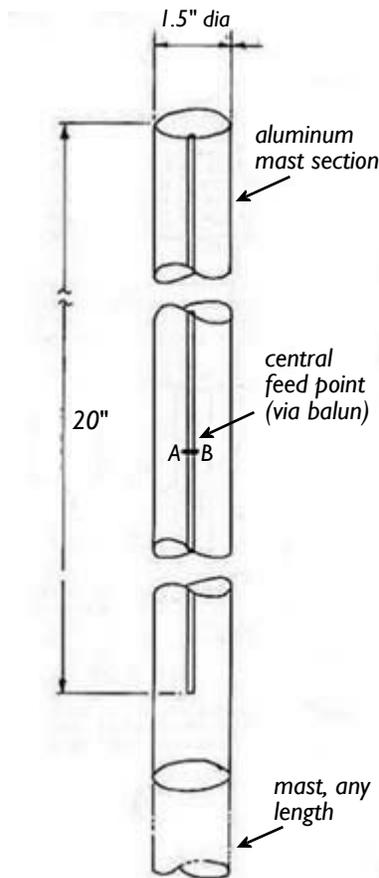
Alford slot antenna for 1.3 GHz designed by M. Walters, G3JVL. Feed impedance across the 11mm wide slot (A-B) is 200  $\Omega$  and requires a 4:1 balun.
