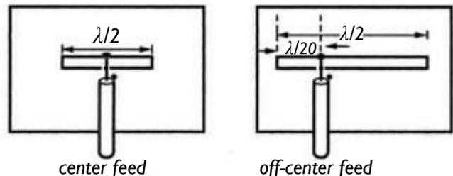
A full-wave slot will match directly to  $50 \Omega$  cable by feeding right at the center.
