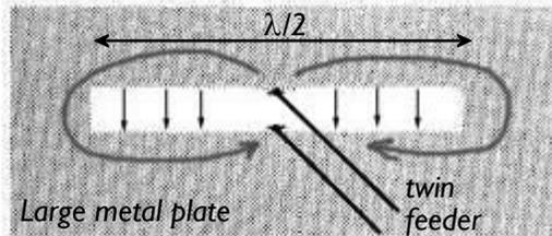
Slot antenna formed by cutting a strip of metal from a large conducting sheet. Arrows indicate the electric field across the slot and circulating currents in the sheet.
