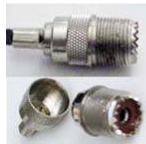
The in-line coaxial connector for RF output just fell apart.
