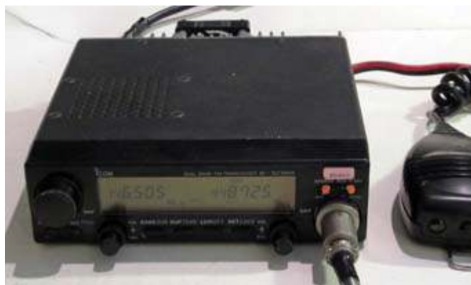
Dark front panel of this Icom IC-3230H was caused by failure of four of the five backlight lamps, leaving only the right-hand POWER button illuminated.
