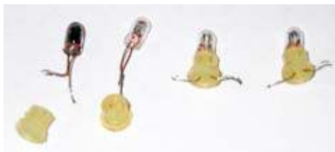
Each of the ‘grain of wheat’ light bulbs was mounted on a silicone rubber sleeve.
