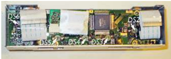
IC-3230H Display Unit board with positions of the five incandescent bulbs DS2 to DS6 arrowed.
