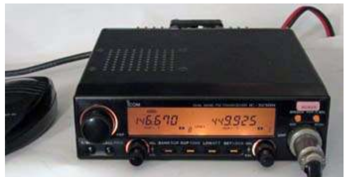
After replacing backlights and cleaning up the radio, the Icom IC-3230H looks almost as good as new.
