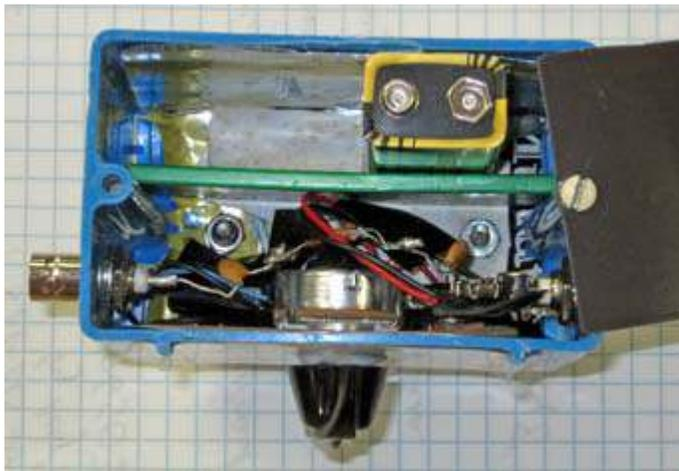
*View inside Lovji's offset attenuator, built inside a blue plastic electrical box.*
