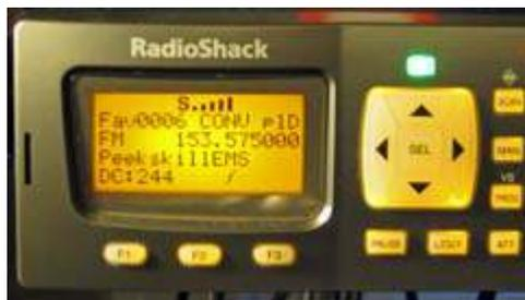
*The LED above the five-way ‘SEL’ pad can be programmed to light in different colors when specific channels are active.*
