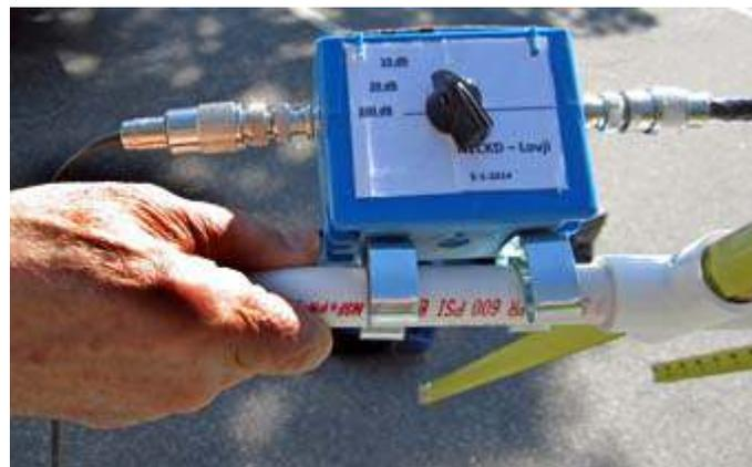
*Offset attenuator mounted on the boom of Lovji's tape-measure Yagi antenna, using steel clips.*
