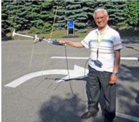
Lovji, N2CKD demonstrates his offset attenuator, which is connected between the tape-measure Yagi antenna and the handi-talkie.
