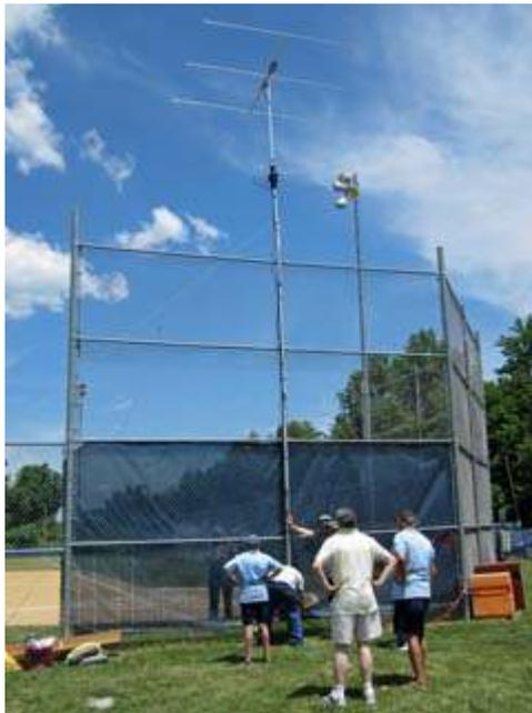
*Yagi antenna plus rotator for 6 meters is pulled up against the wire mesh fence.*
