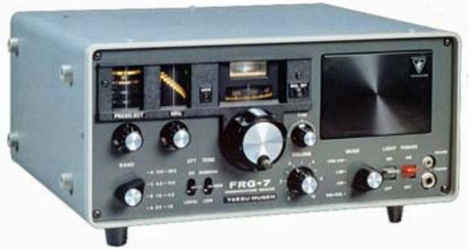
*Yaesu FRG-7 communications receiver from 1977 also employed the Wadley loop for frequency control.*
