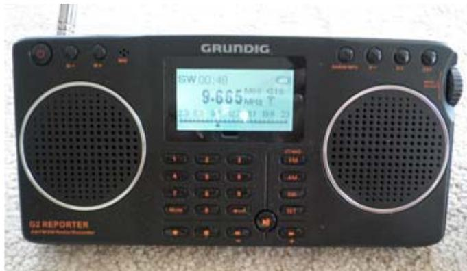
*Grundig G2 Reporter AM/FM/SW receiver with signal strength indicator, MP3 and WMA decoding and recording.*
