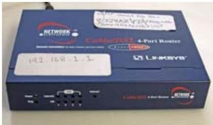
*The FD logging software suffered problems after this Linksys NR041 router overheated and continuously reset itself.*
