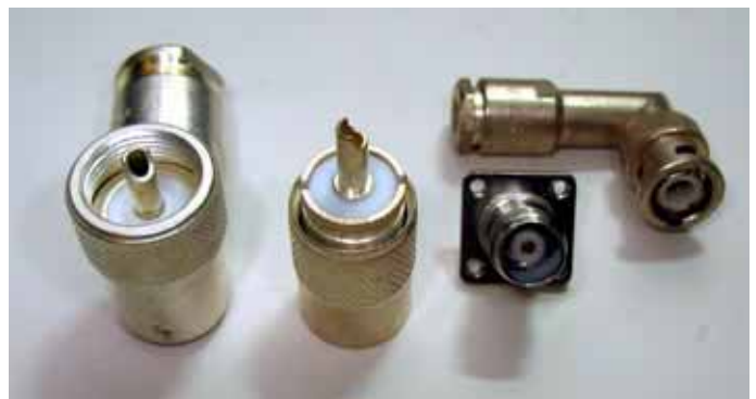
High quality coaxial connectors employ PTFE as the low loss dielectric between inner and outer conductors.
