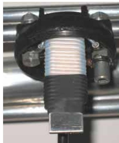
Balun in J-Beam Yagi antenna employs PTFE-insulated wire wound on a metal form.
