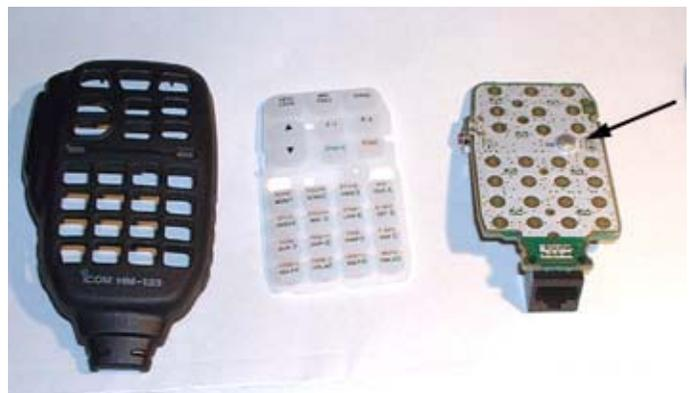
*HM-133 hand microphone from Icom IC-2720 transceiver. Arrow shows the electret capsule mounted on the circuit board.*
