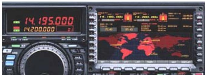
Modern radios, like this Yaesu FT DX 9000D, depend on one or more liquid crystal displays to present frequency and transceiver status information.
