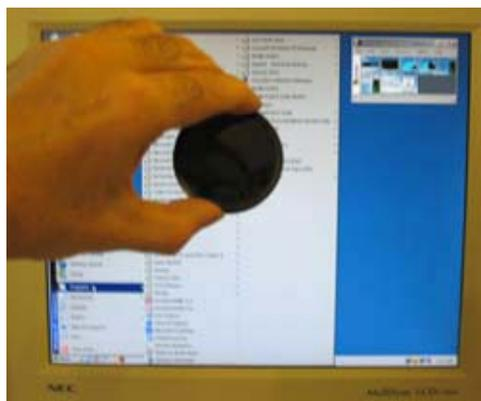
*Rotating a photographic polarizing filter in front of the screen shows that this liquid crystal computer display emits polarized light.*
