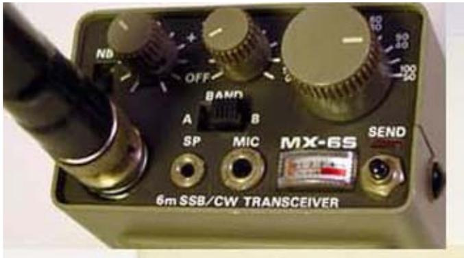
*Santec MX-6S 6 meter SSB/CW transceiver.*
