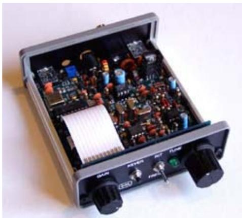
*Small Wonder Labs DSW-II CW transceiver runs 5 watts output on 20 meters.*
