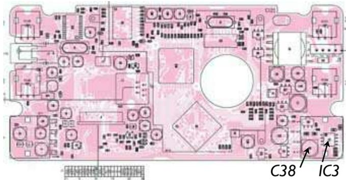
'Control Unit - Bottom View' shows the position of C38 and IC3 (arrowed) on the back of the circuit board.
