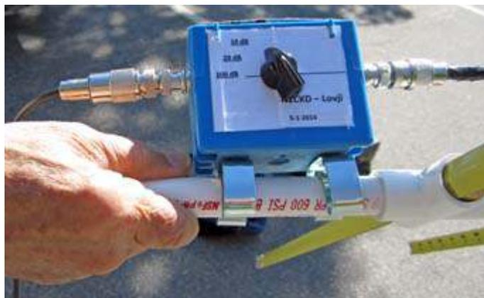
*Lovji's offset active attenuator and tape measure Yagi.*
