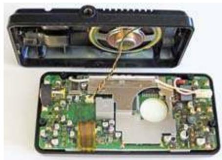
Control head with rear cover removed.
