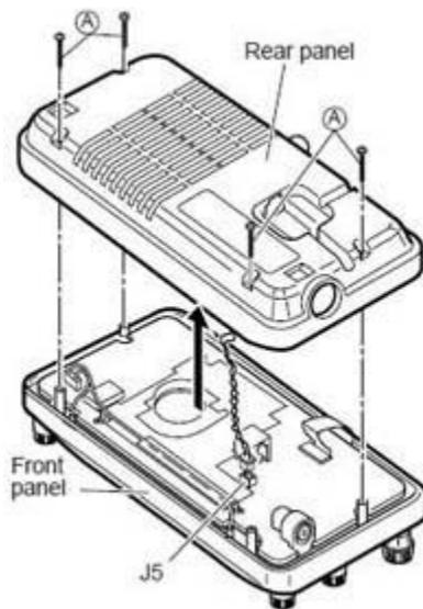
Control head disassembly.
