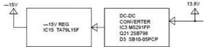
Block diagram shows function of IC3, the DC-DC converter and IC15 the negative 15 volt regulator.
