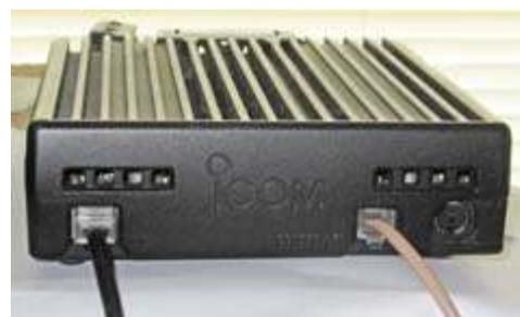
*New, pink cable on the right connects IC-2800H main unit to the control head.*
