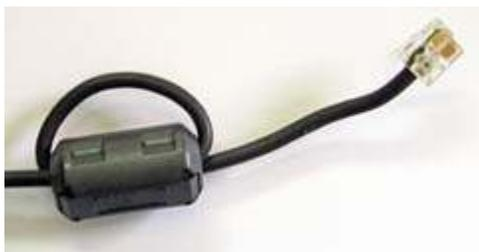
*Icom’s multi-way cable from IC-2800H main unit to the control head has a ferrite core and six-way RJ-11 jack at the controller end.*
