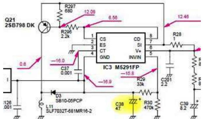
Circuitry of the IC-2800 DC-to-DC converter, with voltage measurement points arrowed. Yellow highlight shows C38.
