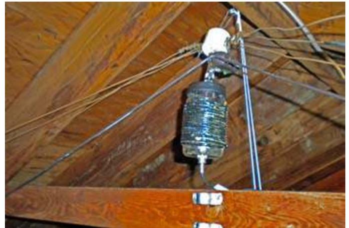
Center insulator and coiled-coax balun for Lovji's multi-band dipole antenna are suspended in the attic. [N2CKD pic.]
