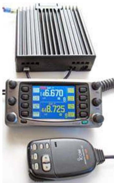
*Icom IC-2800H VHF/UHF transceiver has a large color display on the control unit.*
