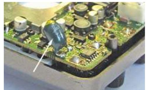
**C38** was replaced by a green-colored 33 $\mu$ F tantalum capacitor (arrowed).
