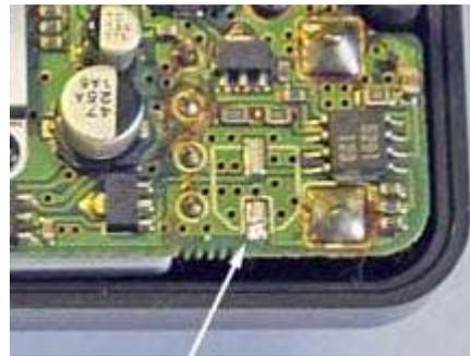
Close-up of the controller board after removal of **C38** (position arrowed).
