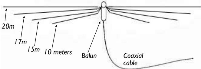
Fan dipole antenna for 14, 18, 21 and 28 MHz has separate half-wave wire dipoles for each of the four bands, all connected to a common feed point. (Note: wire lengths for resonance can be affected by proximity to the other dipoles.)
