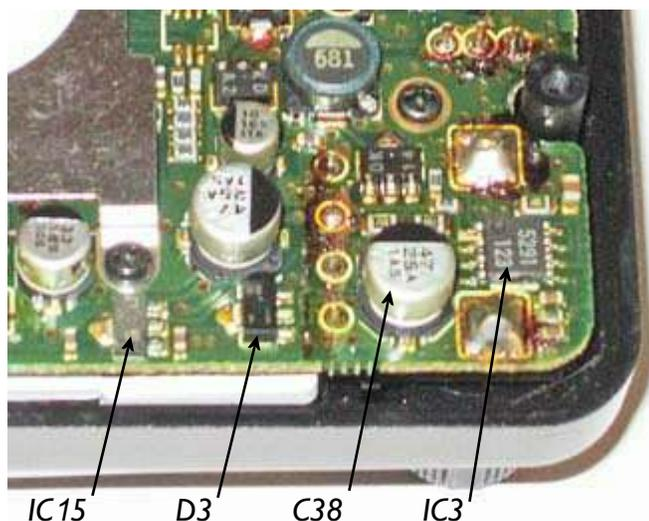
Close-up of the controller board, with components of the -15V regulator and DC-to-DC converter arrowed.
