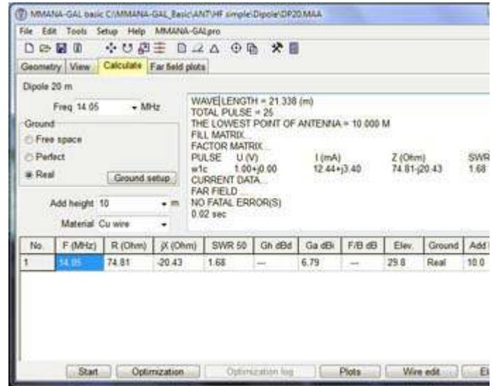
‘Calculate’ tab of the MMANA-GAL program shows the results for a 20 meter dipole after the ‘Start’ button has been pressed. SWR for 50 ohm feeder is 1.68:1.
