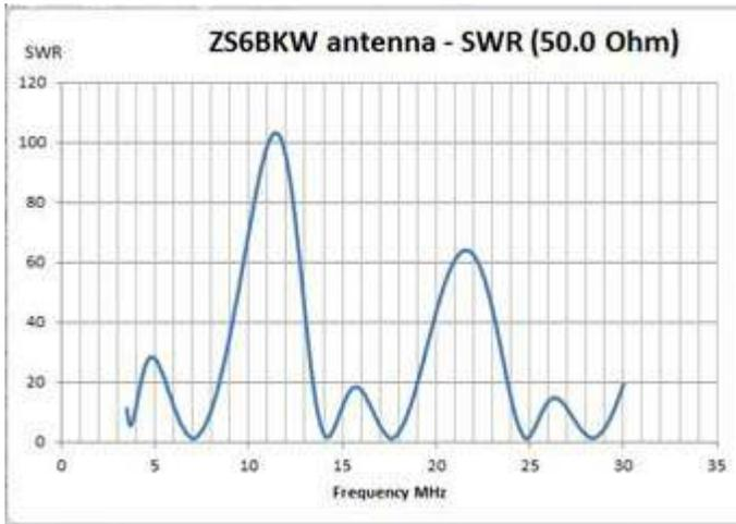
Graph produced by Microsoft Excel from a .csv file generated by MMANA-GAL for a ZS6BKW antenna. Note low SWR on the 3.5, 7, 14, 18, 24.9 and 28 MHz bands.
