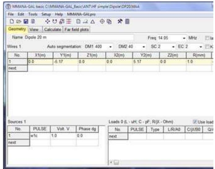
Screen-shot of the MMANA-GAL program at the ‘Geometry’ tab, showing x, y, z co-ordinates of a 20 meter dipole, with lengths expressed in meters. The “Sources” table shows the antenna is fed at the center of wire #1 (w1c).
