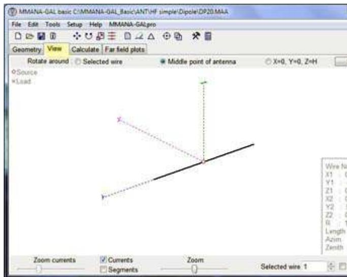
Screen shot of MMANA-GAL program at the ‘View’ tab (yellow tint) shows a horizontal dipole antenna for 20 meters suspended in 3D space.
