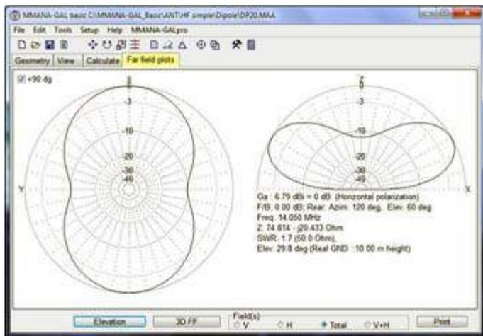
'Far field plots' tab of the MMANA-GAL program shows the azimuth and elevation radiation patterns for a 20 meter dipole, 10 meters above real ground.
