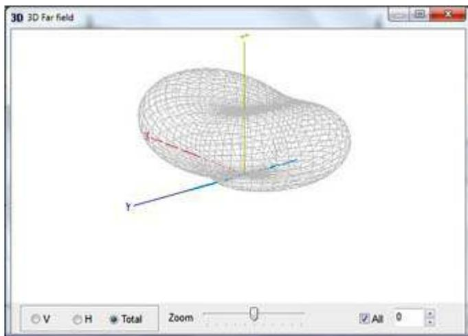
3D Far Field pattern of a 20 meter dipole — as visualized by MMANA-GAL — can be rotated in three dimensions. (The antenna wire is aligned with the Y-axis.)
