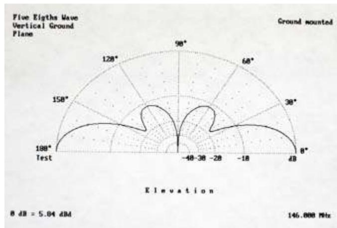
MN software's PLOT program shows the elevation pattern of a  $5/8\lambda$  vertical ground plane antenna on 146 MHz.
